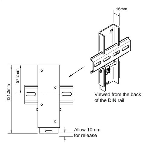
Figure 2-2. DIN-Rail Adapter Bracket
